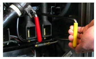
Begin the filtering process by pulling yellow handle to open oil return valve. Leave the drain valve (red handle) open during the filtering process.
